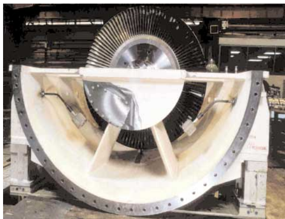
Figure 15. Axial exhaust configuration
