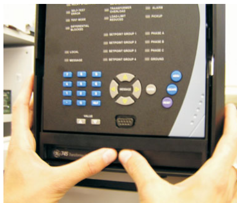
FIGURE 3-5: Press latch to disengage handle
