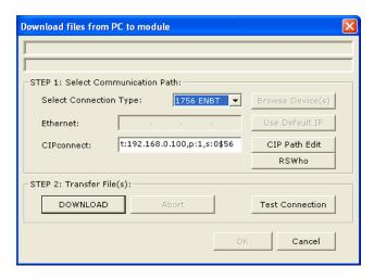
**4** Click **RSWHO** to display modules on the network. The MVI56E-MNETR module will automatically be identified on the network.
