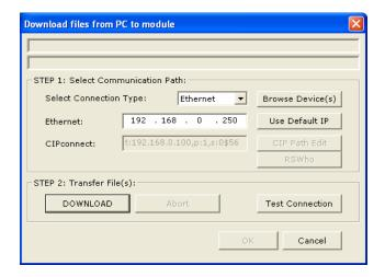
Click **TEST CONNECTION** to verify that the IP address allows access to the module.
