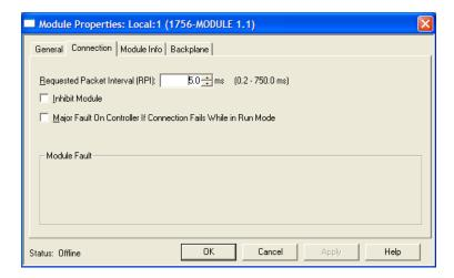
**4** Save the module and click **OK** to dismiss the dialog box. The *Controller Organization* window now displays the module's presence.
