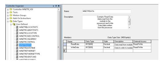
2 Edit the ReadData array size to match or exceed the value of the Read Register Count parameter in PCB.
