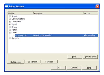
2 Select the 1756-MODULE (GENERIC 1756 MODULE) from the list and click OK. This action opens the New Module dialog box. 3 Set the Module Properties values as follows:
