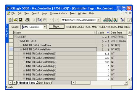
The *WriteData* array is related to the contents of the Write Data area of the module's internal database. To view the actual registers in the module's internal database, access the database display from *ProSoft Configuration Builder's Diagnostics* menu. For more information, see the section on *PCB* Diagnostics (page 83).
