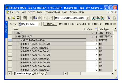
The *ReadData* array is related to the contents of the Read Data area of the module's internal database. To view the actual registers in the module's internal database, access the database display from *ProSoft Configuration Builder's Diagnostics* menu. For more information, see the section on *PCB* Diagnostics (page 83).
