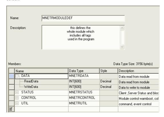
Notice that these UDTs are the data types used to declare the MNETR.DATA.ReadData and MNETR.DATA.WriteData controller tag arrays. Each UDT is commented in the Description column.
