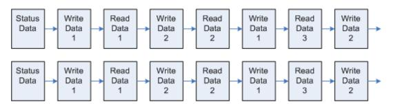
This sequence will continue until interrupted by other special function blocks sent by the processor, by a command request from a node on the Modbus network, or by operator control through the module's Configuration/Debug port.
