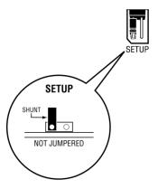
**Note:** If you are installing the module in a remote rack, you may prefer to leave the Setup pins jumpered. You can update the module's firmware without requiring physical access to the module.
