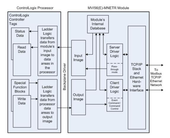
All data transferred between the module and the processor over the backplane is through the input and output images. Ladder logic must be written in the ControlLogix processor to interface the input and output image data with data defined in the controller tags. All data used by the module is stored in its internal database. This database is defined as a virtual Modbus data table with addresses from 0 (40001 Modbus) to 4999 (45000 Modbus).
