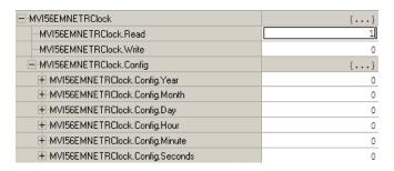
2 The bit will be automatically reset and the current clock value will be copied to MVI56MNETRCLOCK.CONFIG controller tag as follows.
