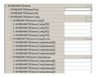
2 The bit will be automatically reset and the current Ethernet settings will be copied to MVI56MNETRETHERNET controller tag as follows.
