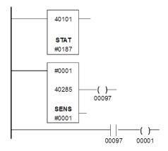
STAT and SENS monitor the I/O status of Drop #2 and inhibit output 00001 if communications are lost. STAT provides access to the system's status, including the status of S908 communications. The status information is stored in a table starting at register 40101 and has a length of 187 words (as shown in the top and bottom nodes of the STAT instruction).
