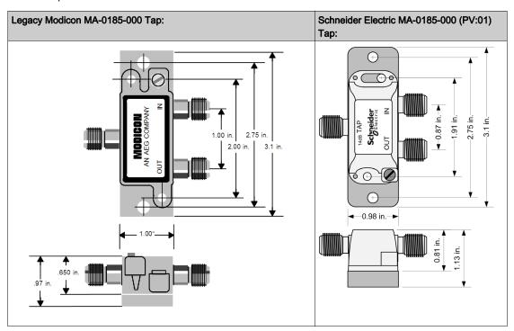
**NOTE:** Although the trunk ports are labeled IN and OUT, these labels can be ignored –it means that the tap is not directional–.
