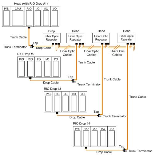
Five chained 490NRP954 fiber optic repeater can be linked in a bus topology. This number can be reduced by the total pulse width distortion (jitter) that occurs on the system (see page 59).
