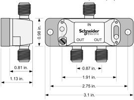
**NOTE:** When not in use, splitter ports must be terminated with a Modicon 52-0402-000 Port Terminator.
