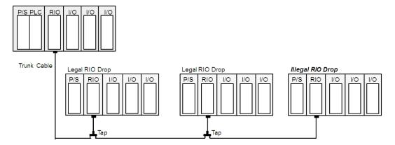
All remote drops on an RIO network must be connected to a trunk cable via a tap and a drop cable, and the last tap on a trunk cable must be terminated with a 75  $\Omega$  Modicon 52-0422-000 Trunk Terminator.
