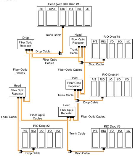
The RIO signal is sent down both legs of the ring by the drop repeater—simultaneously to the head repeaters. A feature is built into the repeaters so that when a signal is received on one of the Rx lines the other Rx channel is blanked—this prevents the same signal from being transmitted twice in the ring.
