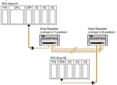
In an optical bus connection, one repeater is always the drop and all other repeaters are heads:
