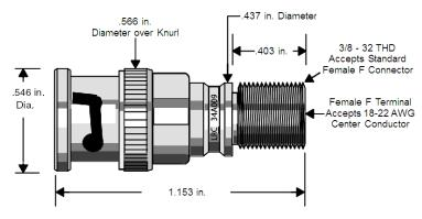
The 52-0614-000 Adapter permits the F connector on an RG-11 trunk cable to be attached to the BNC connector on an RIO processor at the network head-end or the F connector on an RG-11 drop cable to be connected to a J810/J812 or J890/J892 drop adapter at the drop.
