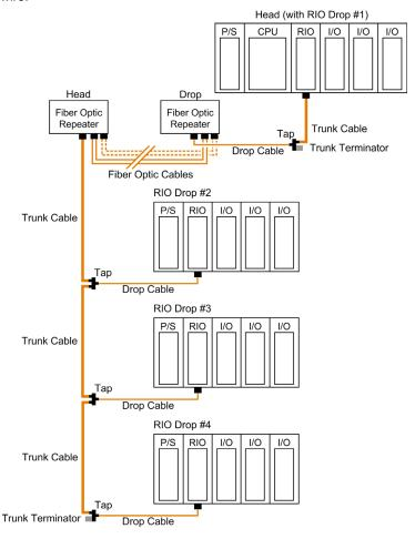
The distance between the two repeaters is limited by the maximum allowable attenuation of the fiber optic cable used in the installation. Fiber attenuation is calculated separately (see page 57) from coaxial cable attenuation.
