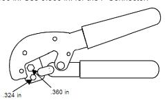
The Modicon 043509432 Crimp Tool is used to install BNC connectors onto RG-6 cable. The tool makes two sizes of hex crimp: 0.276 in. and 0.325 in. Consult Sales, available by special order only.
