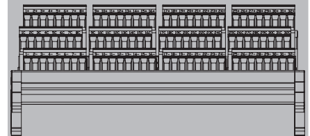
Field terminals view for 1397820000 (ADV151)
