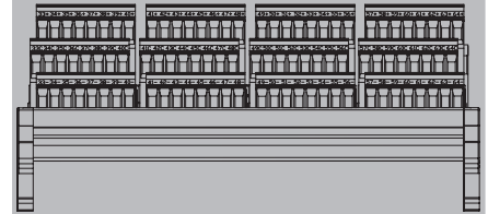
Field terminals view for ADV161 (Channels 33 to 64)
