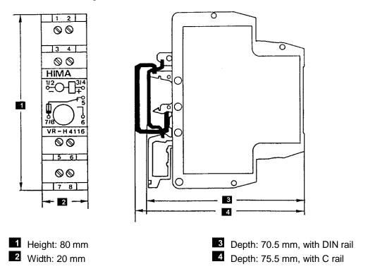
Figure 2: Mechanical Design and Dimensions
