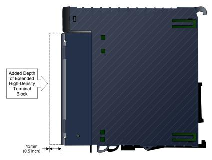
The diagram below compares the space for wiring on a High-Density Terminal Block (left) and an **Extended High-Density Terminal** Block (right), seen from the bottom of the module.
