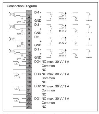
Relays are shown in the unpowered state. The unpowered state is the failure mode.
